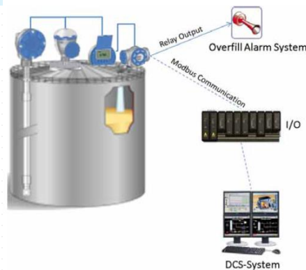
The Raptor two-wire Tankbus requires less cabling.
